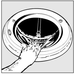
**5** Check the folds in the door seal for any small articles such as buttons or nails which may be lodged there.
